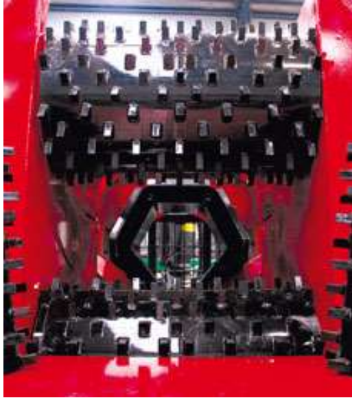
Feeder - With 4 rollers (2 horizontal and 2 vertical) and scrapers to prevent material blockage; great traction power.
