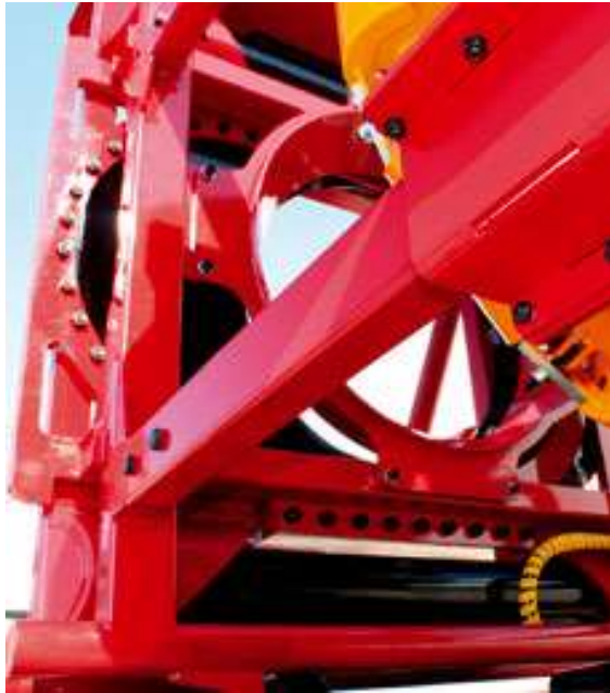
Cutter - Through metal shears (patented system) and with great cutting power; maintenance not required.
