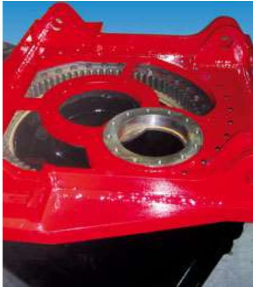
Rotation System - Continuous and unlimited rotation, with 2-stage rotation reducer and oil-bath negative brakes.
