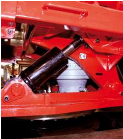
Leveller - 2 powerful hydraulic cylinders control the levelling of the bundler on steep terrain.
