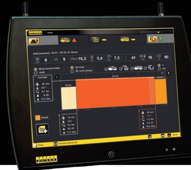
**THE PONSSE ECODRIVE** application provides operators with useful and easily understandable information about the use of the machine. Through the machine's control system, it monitors machine load and fuel consumption for each function and indicates in real time whether the operator's working methods and machine controls are economical and efficient. Eco-Drive lets you focus on what is essential in order to develop working methods.
